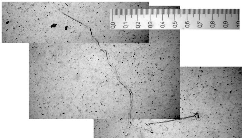
**Fig. 16.** Part of a long (1cm) and irregular track ; scale in mm .
