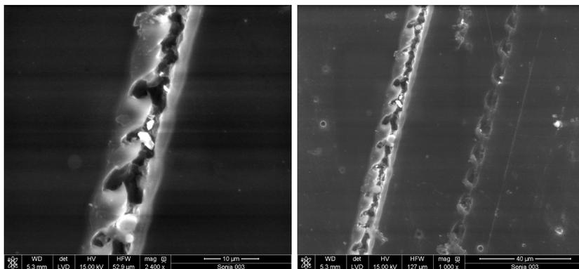
**Fig. 12.** SEM images of the film surface, same track as on figures 8,9; right, detail showing the main track and a secondary one.
