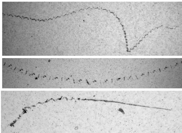
**Fig. 4.** Discontinuous tracks, length (mm) : above 2.4 , middle 2.6, below 1.5 mm.
