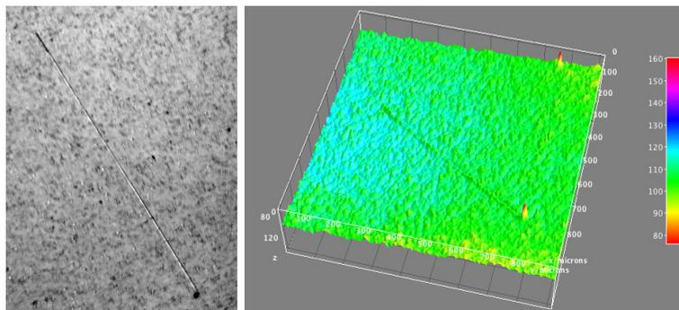
**Fig. 13.** Confocal images of the film surface, left, standard view, right, 3-D reconstruction of the underside.
