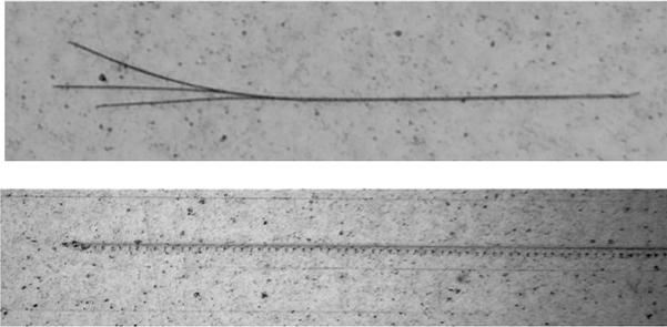
**Fig. 5.** Branching points (length : above 0.77mm, below 1.87mm).
