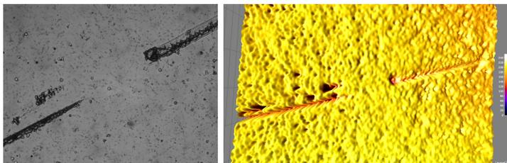
**Fig. 8.** The chosen track, left, with a standard optical microscope, right, surface view with a confocal microscope.
