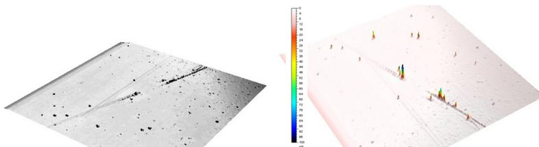
**Fig. 10.** Profilometer images of the film surface, same track as on figures 8,9; right, reversed image showing the underside of the film surface.
